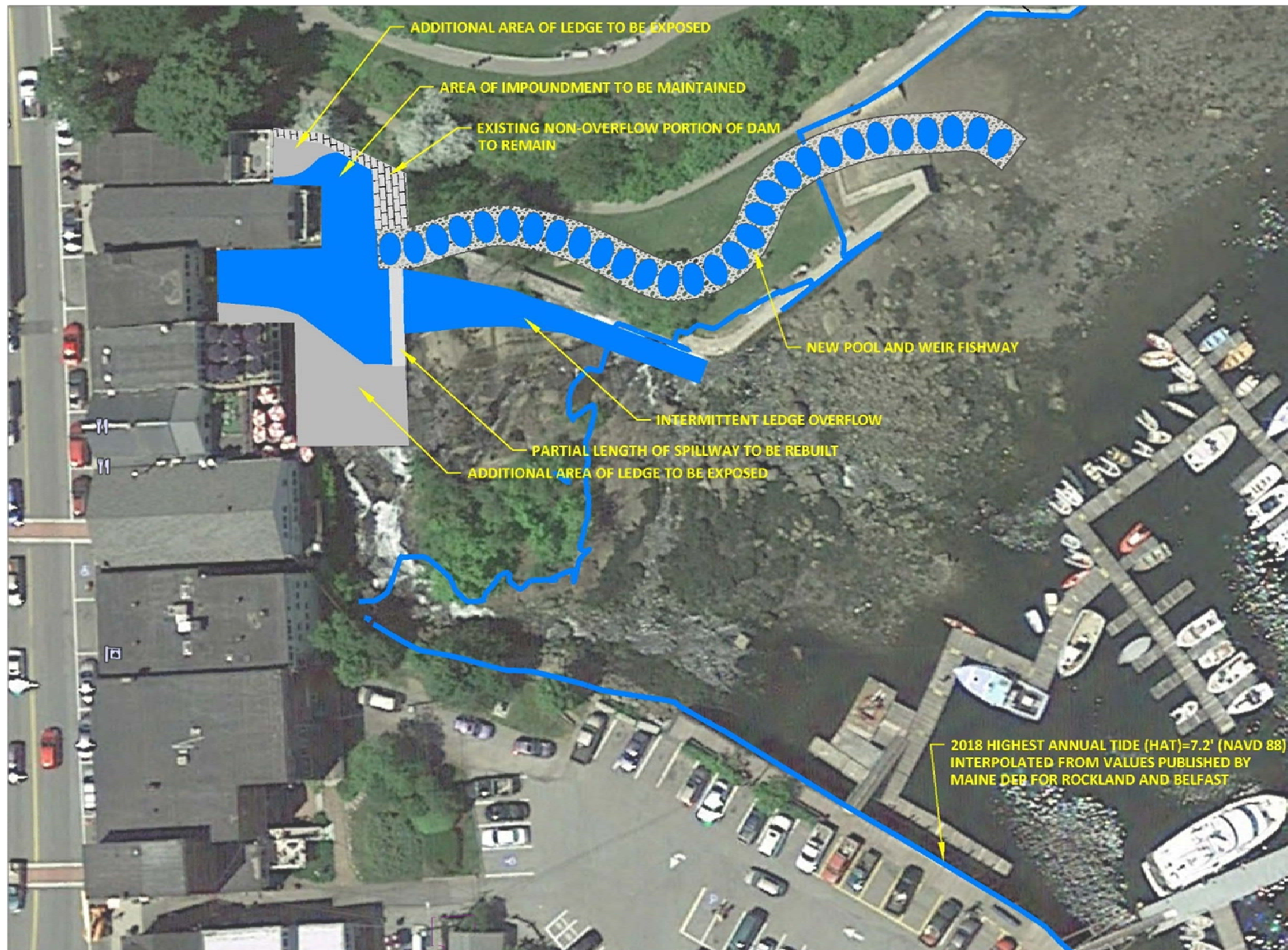
Figure 50. Schematic drawing of partial spillway reconstruction with pool and weir fishway along a conceptual alignment through Harbor Park. Imagery shown represents low tide condition (imagery source: Google Earth).
