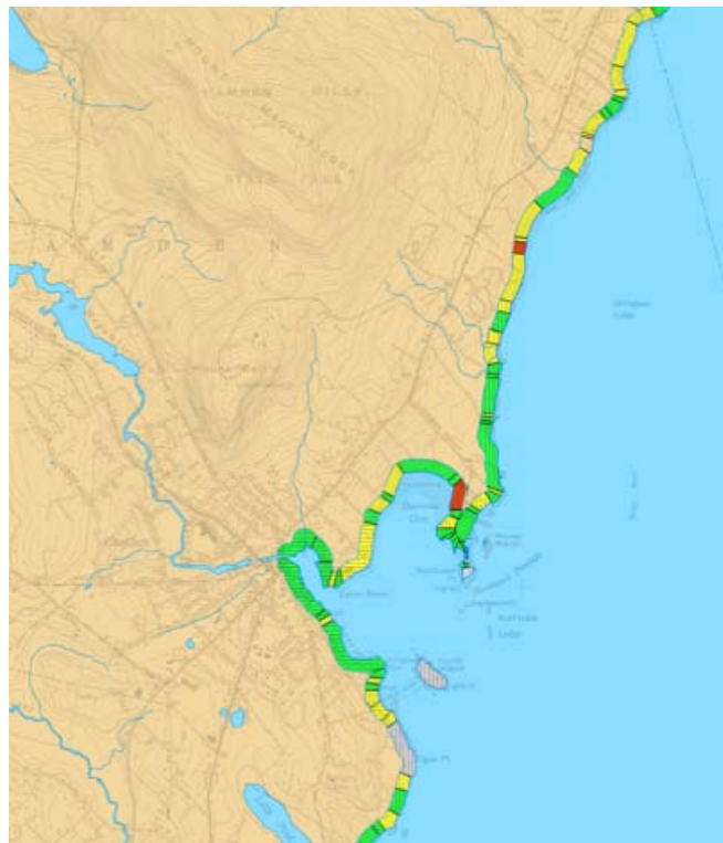
Figure 7. Coastal Bluffs Map for the Camden Quadrangle Grey is rocky shore, Green is stable Yellow is unstable and red is highly unstable.
